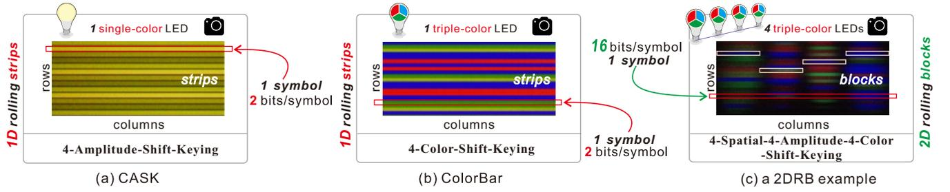
Fig. 1: The illustration of 2D rolling blocks spatial diversity in our proposed (c) a 2DRB example and its comparison with 1D rolling strips spatial diversity in state of the arts in OCC: (a) CASK [1] and (b) ColorBar [2].
