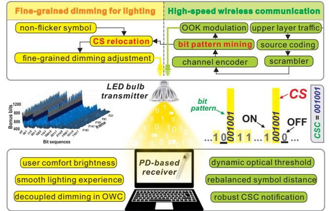
Fig. 2: System architecture and workflow of LiFOD.
