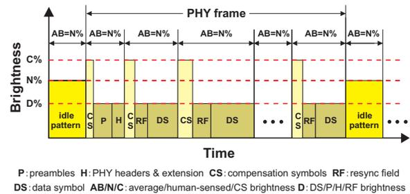
Figure 1: OOK dimming control with CSs [1].
